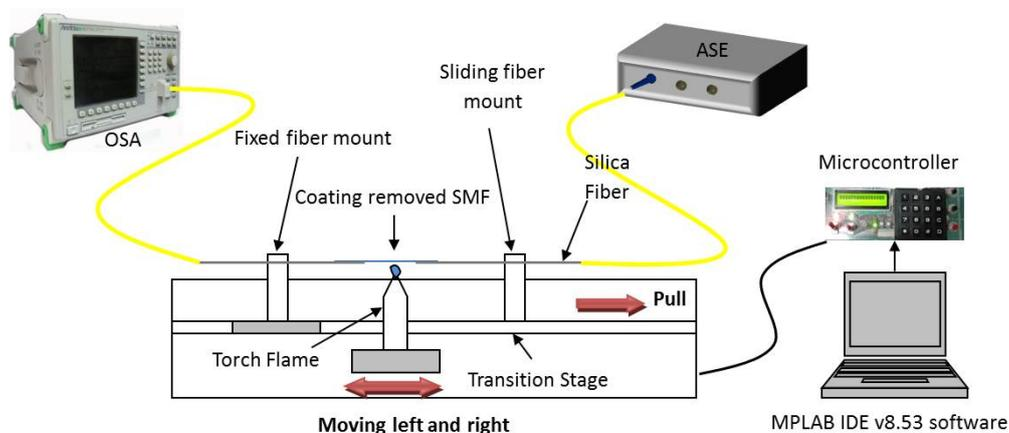
Figure 1: Schematic Illustration of the Silica Microfiber Fiber Setup by Using Flame Brushing Techniques
