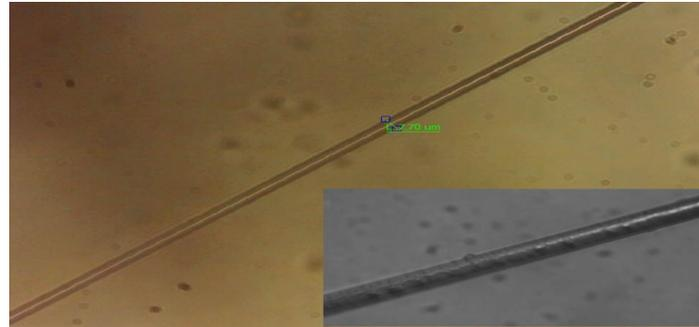
Figure 2: Microscope Image with 20x Magnification of the Tapered Fiber
