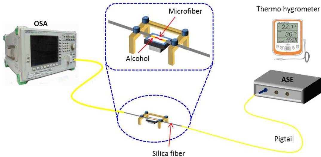
Figure 5: Experimental Setup for the Measurement of Alcohol Concentration Using a PMMA Doped MWCNTs Microfiber
