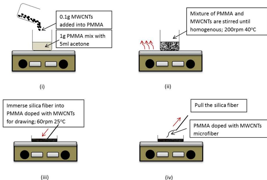
Figure 3: Schematic Illustration of PMMA Doped MWCNTs Microfiber Fabrication Process
