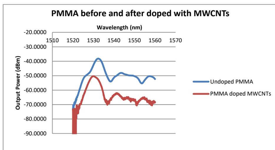
Figure 6: Output Power of PMMA Before and After Being Doped with MWCNTs
