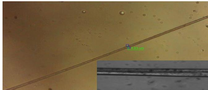
Figure 4: Microscope Image with a 20x Magnification of the PMMA Doped MWCNTs
