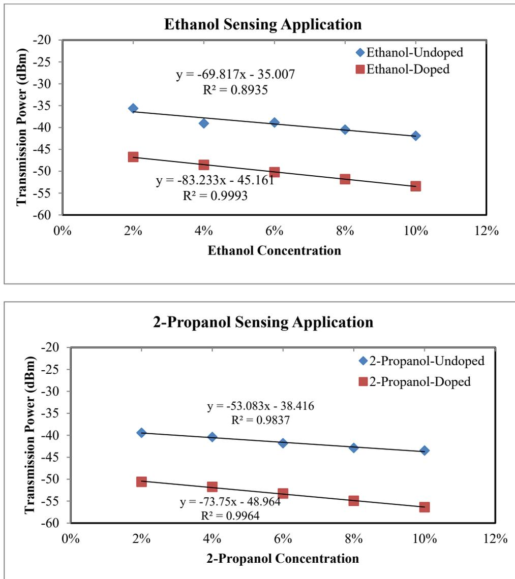
Figure 8: Transmission Output Power for the Detection of Various Kinds of Alcohols at Different Concentration for the Undoped PMMA and PMMA Doped MWCNTs
