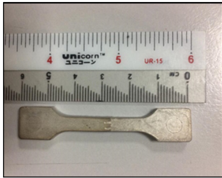
FIGURE 4. Co-sintered part of SS316L and SS17-4PH
