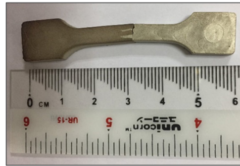
FIGURE 5. Failure in Co-sintering process
