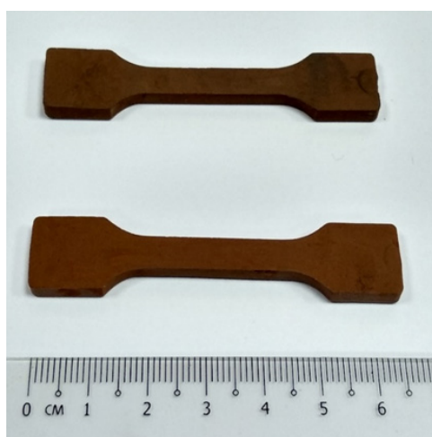
FIGURE 2. Cu 100% and Cu/0.5 vol.% GNPs greenpart
