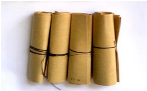
FIGURE 3. The insulating paper being tied before dried
