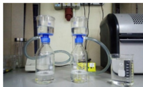
FIGURE 2. Transformer oil filtration
