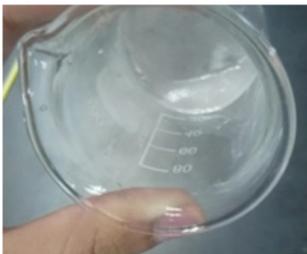
FIGURE 5. Modified PCM in semi-solid state
