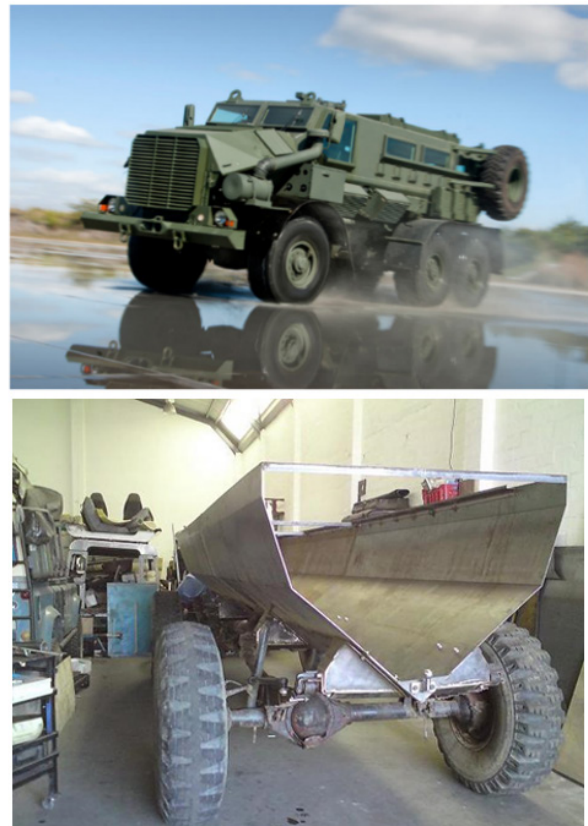
FIGURE 1. An armored personal vehicle manufactured by BAE Systems that utilizes the V-shaped plate geometry Source: Military-Today (2006; Warfare 2018b)
