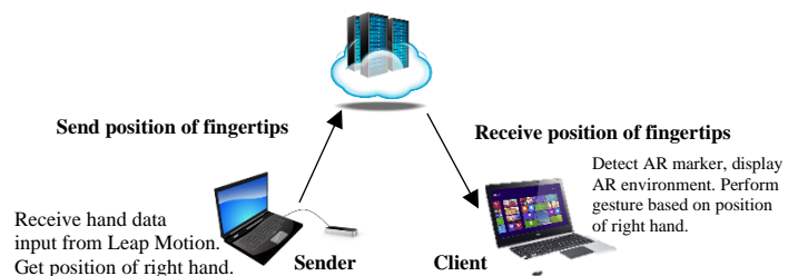
Fig. 13. Flow of the data send by sender and receive with PUN to client [12]
