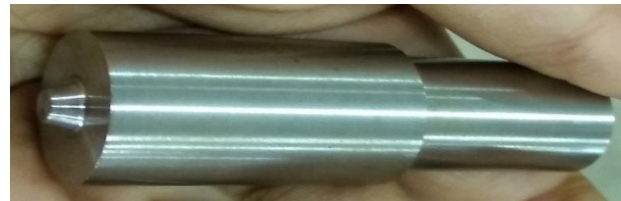
FIGURE.1: H13 grade non consumable tool used for FSP
