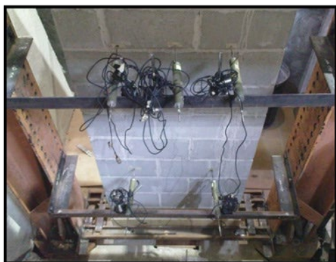
FIGURE 6. Setting Out of LVDT
