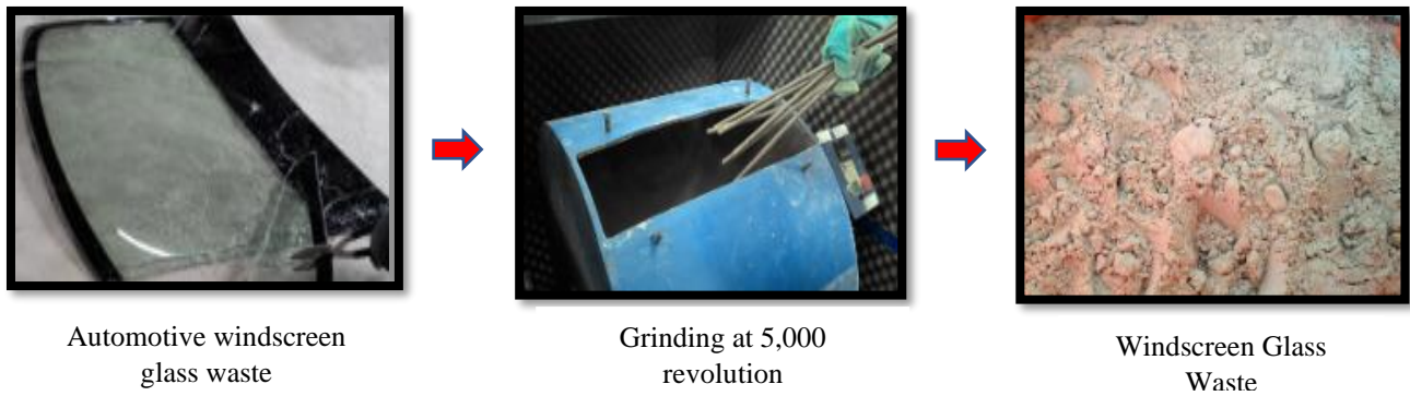
Figure 1. Preparation of automotive windscreen glass waste (WGW)
