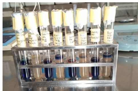
Fig. 1. Biodegradation screening set up of hydrocarbon utilizing bacteria. Tube 1: Has a control tube with BHM, DCPIP and a similar tube with BHM, DCPIP, Engine oil and consortia isolates. Tube 2: Has a control tube with BHM, DCPIP and a similar tube with BHM, DCPIP, PMS and consortia isolates. Tube 3: Has a control tube with BHM, DCPIP and a similar tube with BHM, DCPIP, Diesel and consortia isolates. Tube 4: Has a control tube with BHM, DCPIP and a similar tube with BHM, DCPIP, Kerosene and consortia isolates.
