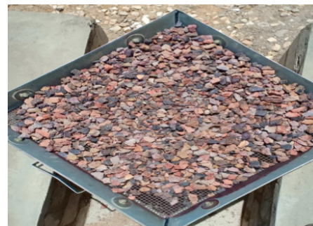
FIGURE 2. Crushed over-burnt brick
