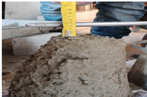
(a) Slump test
