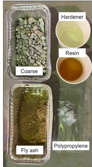
Figure 2. Materials used in the preparation of polymer concrete mixture
