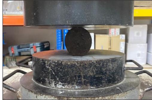
Figure 5. Lateral compression load of polymer concrete
