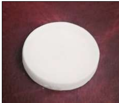
Figure 1. Nb_2O_5 target used for deposition process.
