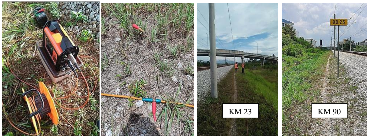
Figure 3: Electrical resistivity conducted at KM 23 Pinang Tunggal and KM 90 Alor Setar station.
