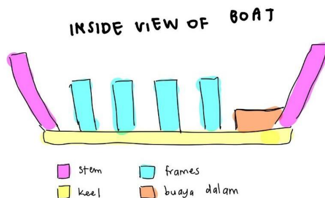
Figure 2: Basic structure of a Terengganu traditional boat.
