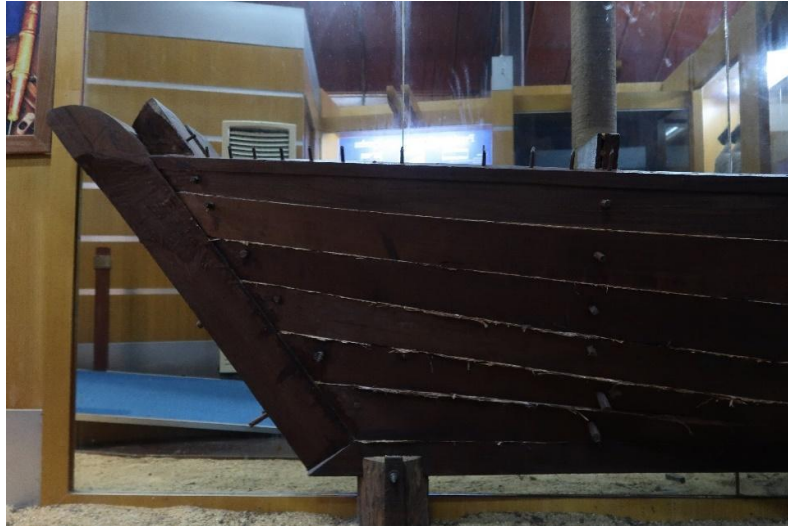
Figure 5: Image of a traditional boat showing cylindrical pasak fixed in the Lepang planks.
