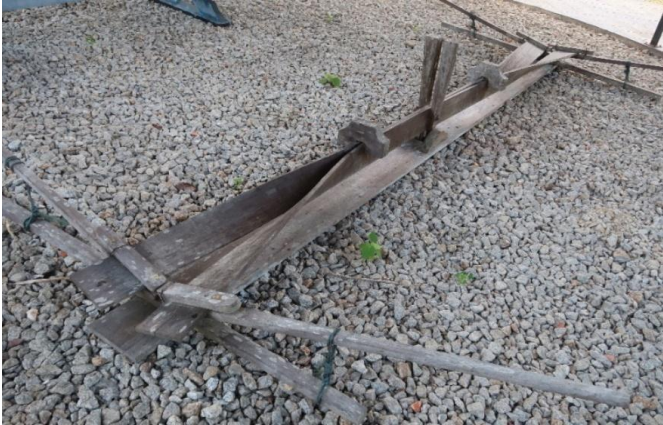
Figure 3: The process of shaping and blending the planks to the basic concave shape of a boat
