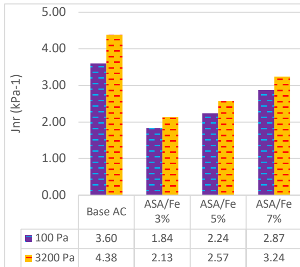
FIGURE 9b. Non-recoverable creep compliance for base, ASA/Si and ASA/Fe composites
