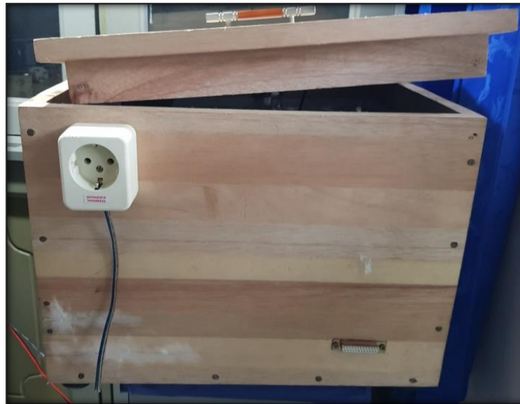
Figure 4: The instrument for testing the effect of the three physical parameters on the output of the photodiode of the self-produced optocoupler.
