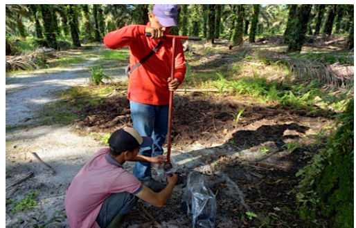
Figure 4. Illustration of soil sampling using auger (Internal documentation of Wilmar Plantation Indonesia, 2023)
