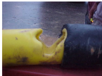
Figure 5 Damaged MDPE gas pipe showing serious shear remnants of sand blasting impact
