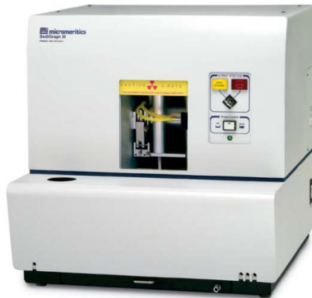
Figure 1 SediGraph III 5120, a commercial version of particle size measurement. Measures particles range from 0.10 to 300 \mu\text{m} equivalent spherical diameter using stokes law [14]
