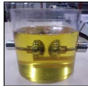
Figure 2 Filling the test cell with test sample
