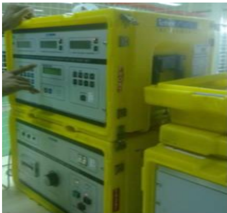
Figure 4 Equipment for dissipation factor measurement
