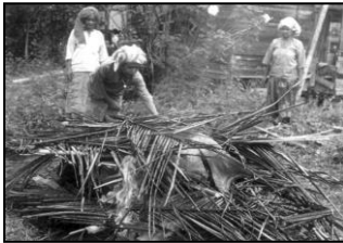
Firing in open trenches
