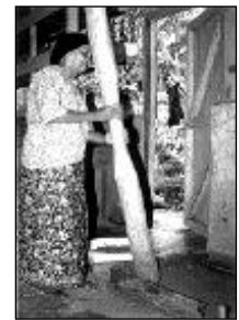
Pounding the clay using wooden hand pestle
