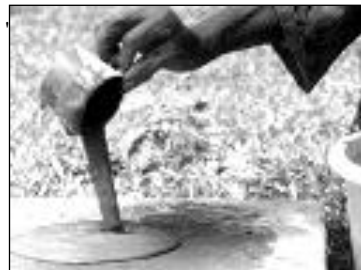
Blending the slip using a plunger
