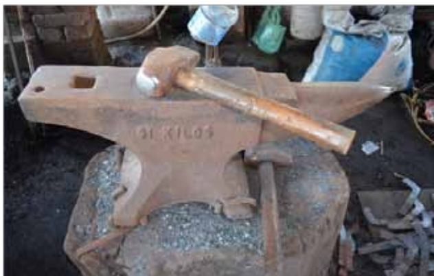
Figure 4 The anvil used by the blacksmith in making iron equipment.
