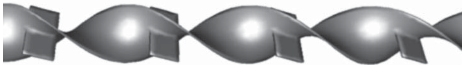
FIGURE 1. Slant baffled twisted tape insert
