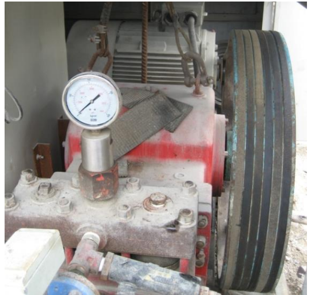
Figure 4 A YBM secondhand high jet pump was modified by the authors
