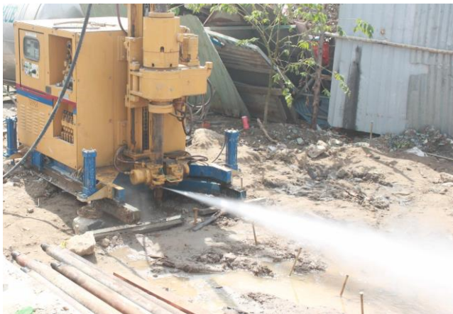
Figure 3 A YBM SI-30S grouting machine employed for this study
