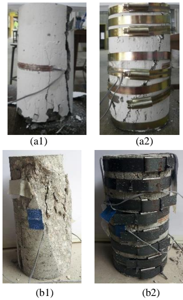
Figure 8 The cracking pattern of (a1) unconfined and (a2) SSTT(HC) confined specimens, (b1) unconfined and (b2) SSTT(SS) confined specimens
