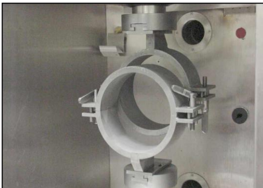
2c. FDOT shear tester [29].
