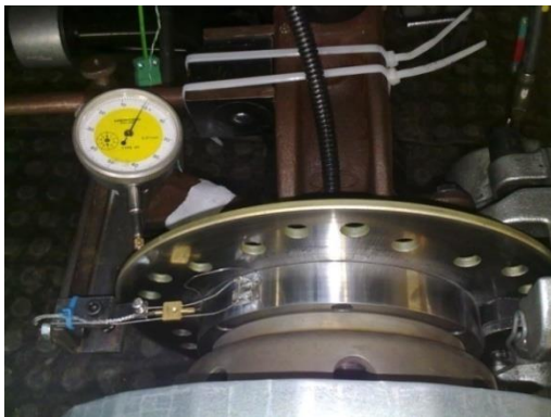
Figure 8 Rubbing thermocouple on the hub of the prototype lightweight disc with a dial gauge to indicate the disc coning deflection
