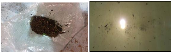
Figure 24 Type of soil and sediment in water tank
