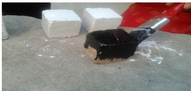
Figure 2 Application of protective coatings
