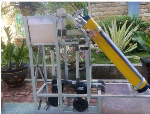
Figure 2 Turbine screw experimental apparatus
