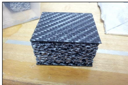
Figure 1 Closed-cell aluminium foam with CFRP composite sandwich panel
