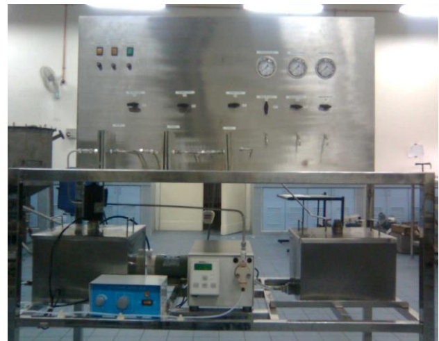
Figure 2 Filtration system with plates and frame filter cells
