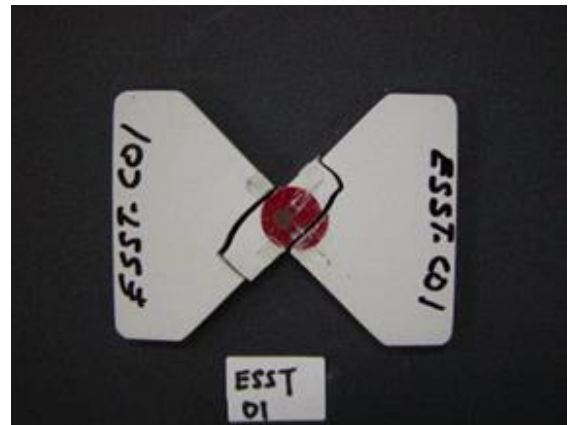
Figure 9 Brittle failure of ESST-C01 occurred in \pm 45^\circ plane
