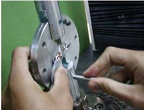
Figure 7 Attachment of grip to holder by pin
