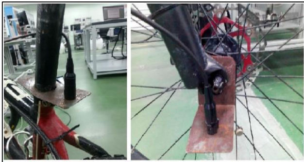
Figure 2 Sensor placement: Seat post (left) and front fork (right).
