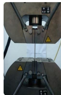
Figure 4 Test sample undergoing tensile test
