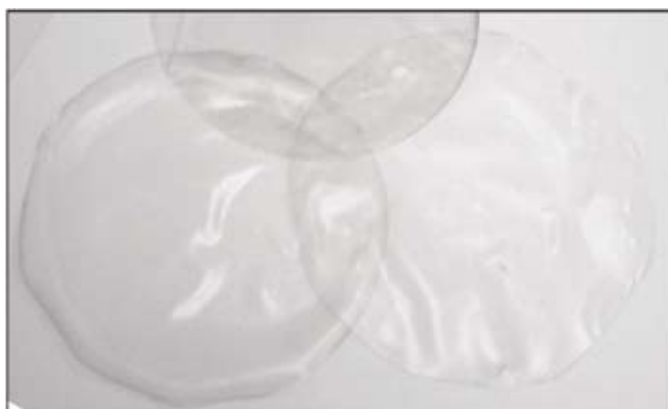
Fig. 4: A translucent starch-based film incorporated with lysozymes
