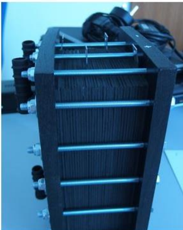
Figure 1 Complete built up of the alkaline electrolyser (left) and schematic diagram of the cell (right)
