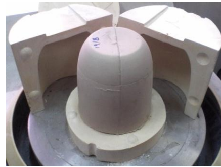
Figure 2 De-moulding of hollow product
