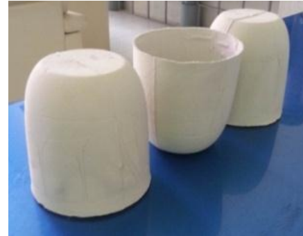
Figure 3 Dry green body of hollow products
