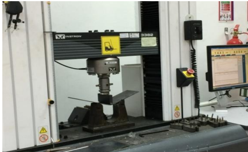
Figure 2 Three-point bending process
