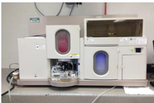
Figure 3 Atomic absorption spectrophotometer for TCLP test
