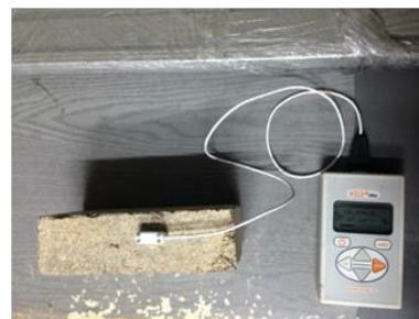
Figure 2 KD 2Pro devices for Thermal conductivity test
