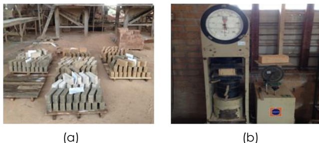
Figure 1 (a) Industrial scale brick samples (b) Compressive strength test for bricks
