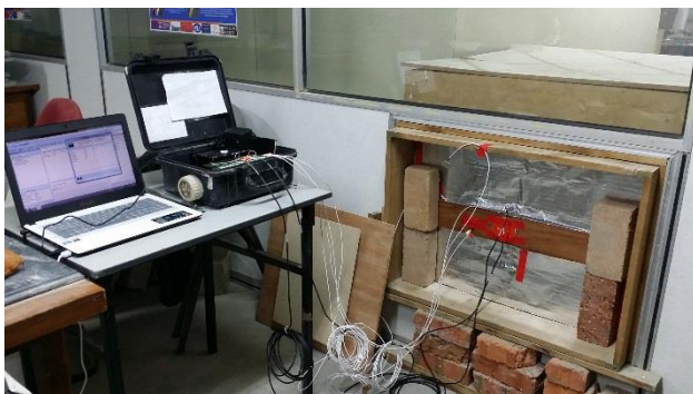
Figure 4 Connection of sensors from the hot box setup to data logger
