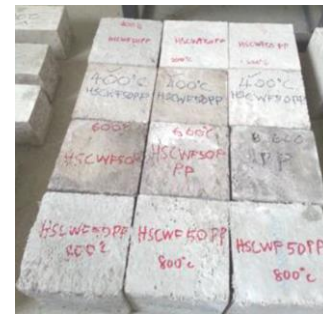
Figure 3 Condition of concrete specimens with PPF after exposed to elevated temperature
