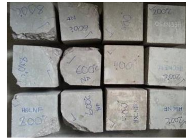
Figure 4 Condition of control concrete specimens after exposed to elevated temperature
