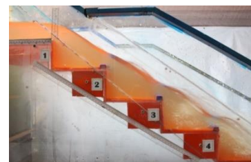
Pooled steps spillway
