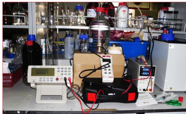
Figure 1 Photograph of MEC system used in this study, with power sources, benchtop multi-meter, water bath, water displacement gas collecting system, conductivity meter
