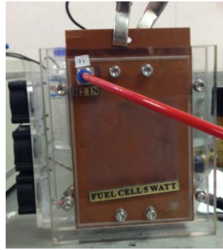
Figure 4: The 5 watt PEM fuel cell stack
