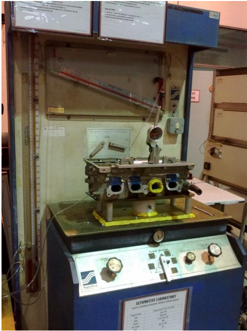
Figure 1: SF600 FlowBench machine with tested cylinder head
