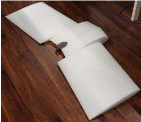
Figure 4. The fuselage and wing parts produced by the CNC hot wire cutter machine.
