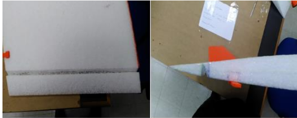
Figure 8 Elevon control surface for the Neo-Ptero \mu -UAV model
