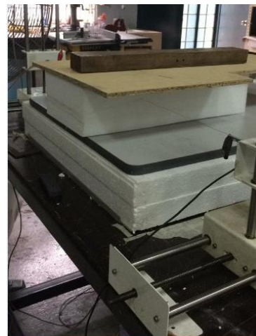
Figure 3 CNC hot wire cutter machine at IFCON (M) Sdn Bhd.
