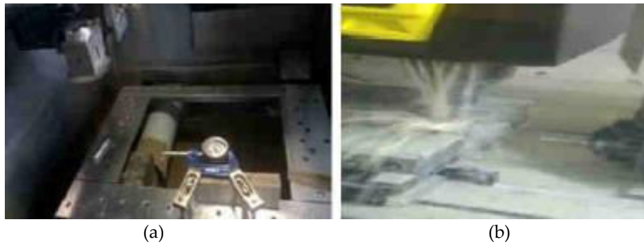
Figure 1: Mould machining process: (a) Wire cut machine and (b) CNC milling
